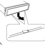
The frame can be removed from the bottom side in the same manner.
